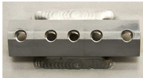
Figure 4.6: Rail welded to the JET vacuum vessel for remote handling positioning and mounting of diagnostic assemblies [3].
