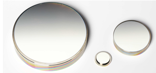
Figure 7.10: 17.5 mm, 50 mm and 100 mm \text{SiO}_2/\text{TiO}_2 dielectric coated mirrors on 1.4429 stainless steel substrate used in the testing.
