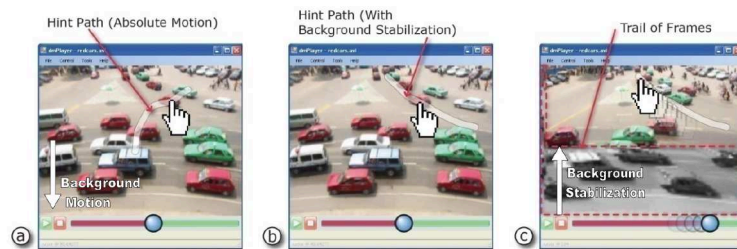
Figure 2.7: DimP allows direct manipulation video navigation even when the camera is moving by shifting the position of the image in the video view in the opposite direction of the camera movement. From [Dragicevic et al., 2008]
