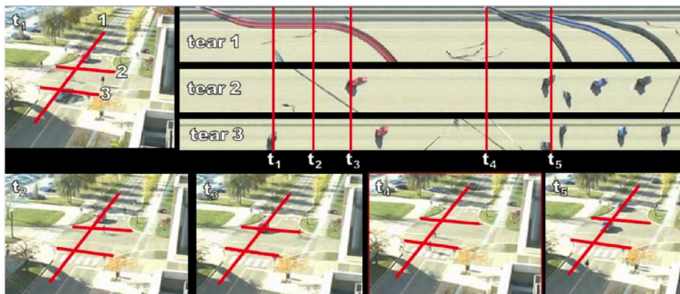
Figure 2.5: SlitTears replicate the pixels under lines drawn in a video scene on a timeline. When the pixels change this creates visible effects on the timeline that can be interpreted by the user, e.g., the long curved streak in tear 1 indicates a car coming from the top stopping at the intersection and then continuing. From [Tang et al., 2009]
