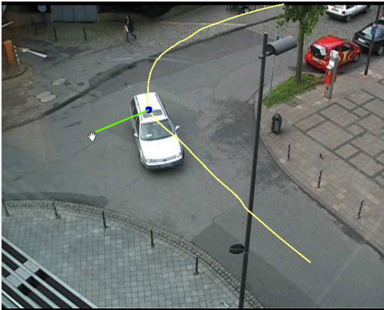
Figure 1.6: Video navigation using the DRAGON interface [Karrer et al., 2008]. Users can select objects such as the car by clicking. The system shows the movement trajectory (yellow) and allows her to navigate in the video by dragging to a specific location. The object will snap to the time where the location on its movement trajectory is closest to the mouse cursor.
