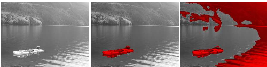
Figure 4.1: Example of an unsupervised segmentation. Having in mind that no prior knowledge is given and the only feature the algorithm deals with is a gray-value distribution, segmentation results can sometimes seem meaningless to a human observer, while still correct based on the presented criterion. Images respond to the original image, the ground-truth segmentation and a result of our method, respectively.
