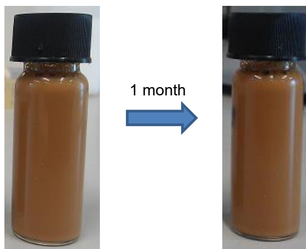
Figure 4.17 Cu@AgNPs after the synthesis (left) and after the one-month storage on the air (right)
