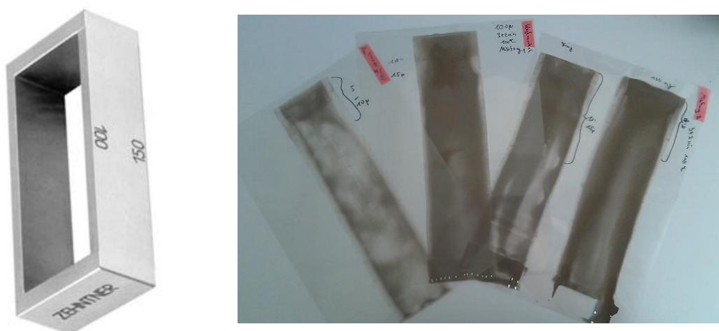
Figure 4.34 Frame for film building (left) and the composite films on PET substrate (right)
