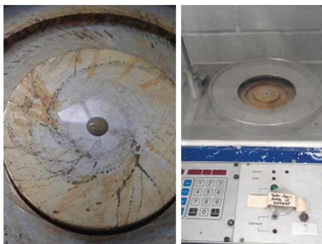
Figure 4.32 Hybrid microgel ink on the glass substrate (left) and the spin coating device (right).
