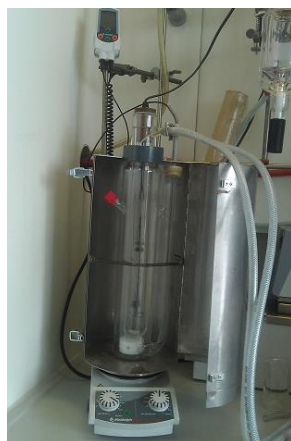
Figure 4.7 UV reactor. Heraeus Noble UV-RS-4 700 W
