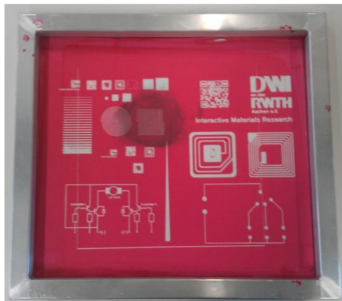
Figure 4.35 Frame for the screen printing.
