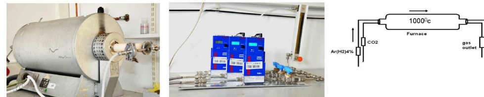
Figure 4.7: A picture of the tube furnace used to synthesize the polycrystalline samples, flow controller and schematic diagram of the furnace respectively.
