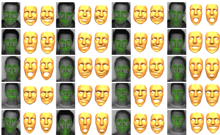
Figure 7.5.: Results produced with our system. Each block contains an image of the video sequence (left), the result produced with our system (middle) and the corresponding 3D stereo reconstruction as a ground truth comparison. The results of our system are quite similar to the baseline.
