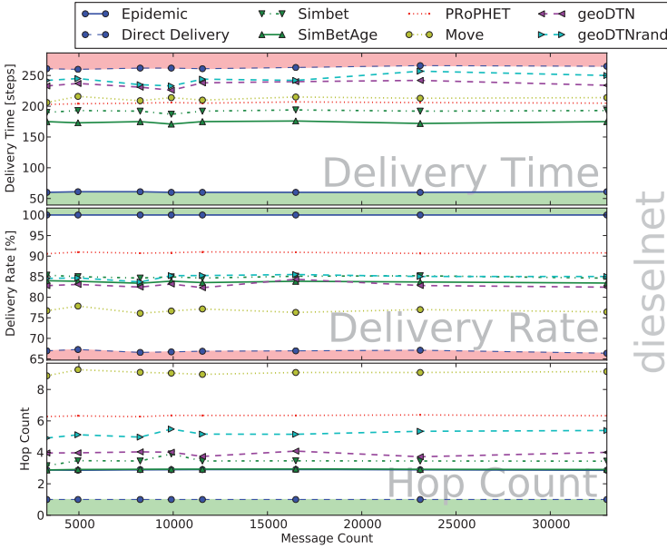
Figure 6.2 Evaluation of the delivery time, delivery rate, and hop count in UMass DieselNet.
