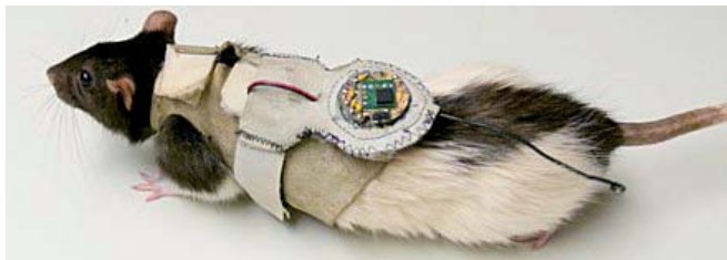
Figure 2.6 Norway rat equipped with sensor node. Our first prototype was based on the mica2dot sensor node, sending data using a low-power CC1K based radio in the 433 MHz part of the ISM band. Later prototypes operated based on the CC2420 radio in the 2.4 GHz band.
