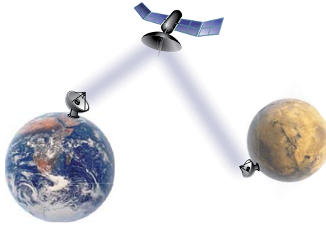
Figure 3.5 An example for a high delay, interplanetary network. A rover on Mars collects data and measurements. Once an orbiter—whose orbit is known in advance—is in range, the rover forwards the data to the orbiter. As Earth becomes visible to the orbiter, it forwards the data to receiver stations on Earth. Due to the speed of light, a message will take between 3 and 21 minutes to reach Earth. However, this delay is very predictable.
