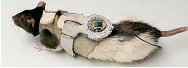
Figure 7.6 Norway rat equipped with the initial mica2dot based sensor prototype.
