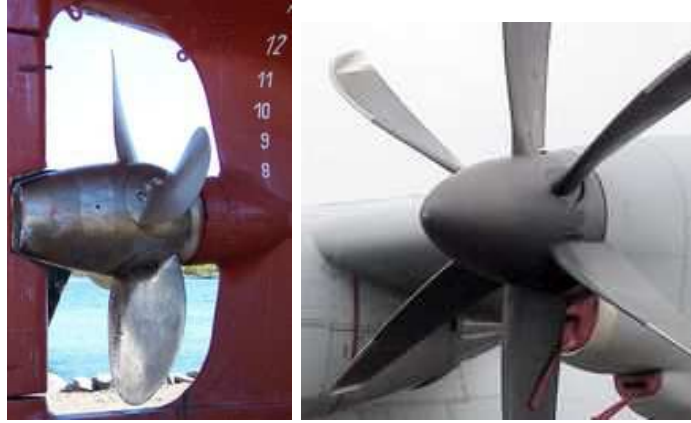
Figure 5.4: Controllable pitch propellers of a Hurtigrutenschiff and a Hercules aircraft propeller [Car07].
