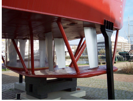
Figure 5.2: Voith Water Tractor propulsion system [RV05].
