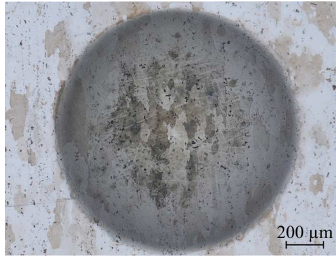
Figure 6.19: The size of a sphere indent relative to the size of the grains of aluminium 2024-T351.
