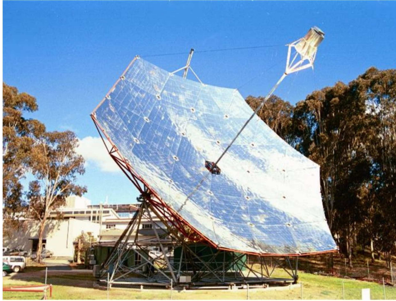
Figure 2.4 The Big Dish prototype at the campus of the Australian National University [56].
