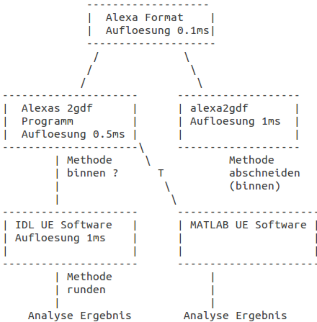
Figure 2.4: Illustration of the data preprocessing workflow, taken from the 1997 report of MD (in German) on the comparison of the first UE implementation in IDL (left branch) and the second implementation in Matlab [69] (right branch). Data entering both analysis branches have a resolution of 0.1 ms (top box). In the IDL branch spike times t in the original data are first transformed to a resolution of h = 0.5 ms (by the 2gdf program, middle left) using the method of binning \lfloor t/h \rfloor . Then the data are read into the "IDL UE Software" (lower left box) and therein converted to h = 1 ms resolution by the method of "round half up" \lfloor t/h + 1./2 \rfloor prior to analysis. Alternatively, one can load the 0.5 ms resolution data into the "MATLAB UE Software" (lower right box). Here the bin width is a parameter of the analysis and thus data can be converted to a 1 ms resolution but results are different from the IDL branch. Results are only identical if a prior transformation "T" (diagonal in center) performs a round half up and no further binning is done in the MATLAB program. At a later point in time the alexas2gdf converter function (written in MATLAB) became available such that data in the original 0.1 ms resolution could directly be converted to the 1 ms resolution by binning.
