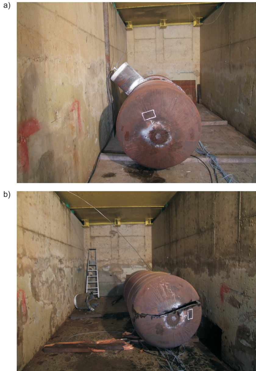
Figure 7.28.: The pressure vessel in the burst cavern a) before and b) after the burst test.
