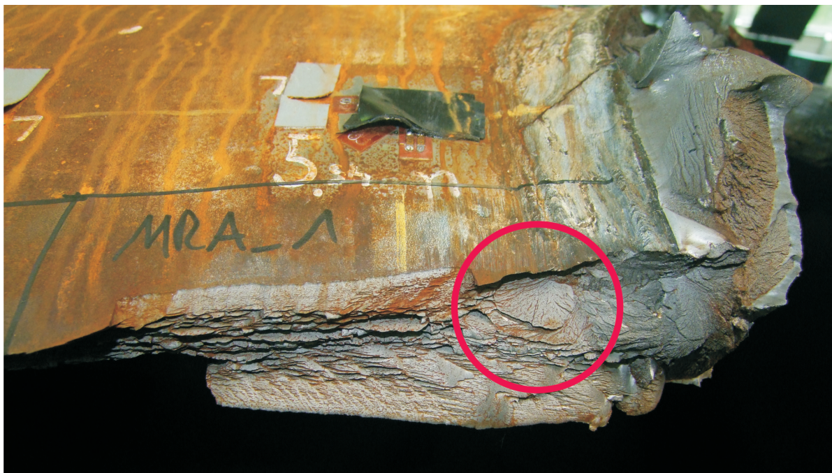
Figure 7.36.: Probable initiation site of failure. The fan-like structure in the HAZ of the weld seam, marked by the red circle, is the suspected crack origin.
