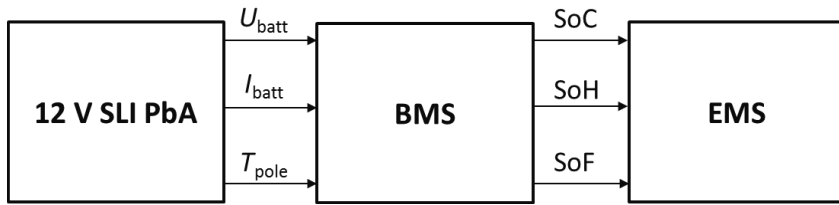
Fig. 2. Simplified graphic representation of BMS functionality in \mu H applications.
