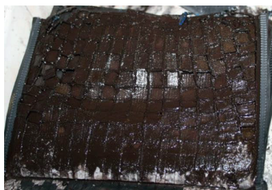
Fig. 115. Considerably corroded positive plate withdrawn from the short-circuited cell of a failed 74 Ah standard flooded SLI battery.
