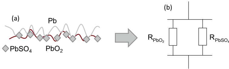
Fig. 113. Schematic illustration of the expected contact surface forming short-circuits between positive electrode and negative COS: (a) schematic visualization of the expected contact surface, (b) equivalent electrical circuit of R_{\text{film}} .
