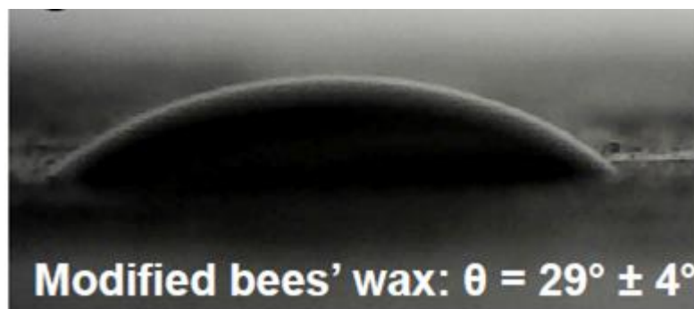
Figure 34: Snapshot of the contact angle of erucamide modified bees' wax on a glass coverslip. Very low contact angles of around 29° can be achieved.
