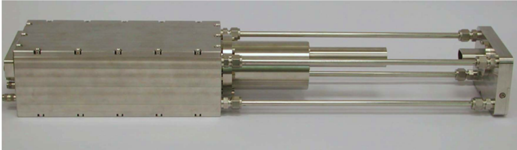
Figure 2.1: The detector head with the movable tube (source: [9])
