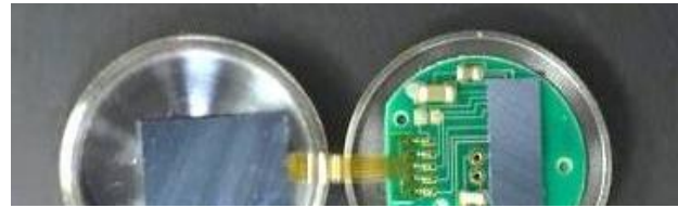
Figure 6: View inside the metal housing of the pressure sensor system with integrated components.
