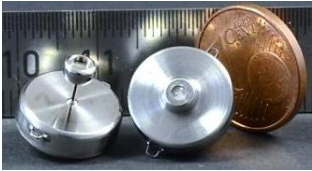
Figure 8: Final design of a welded pressure sensor system for venous application
