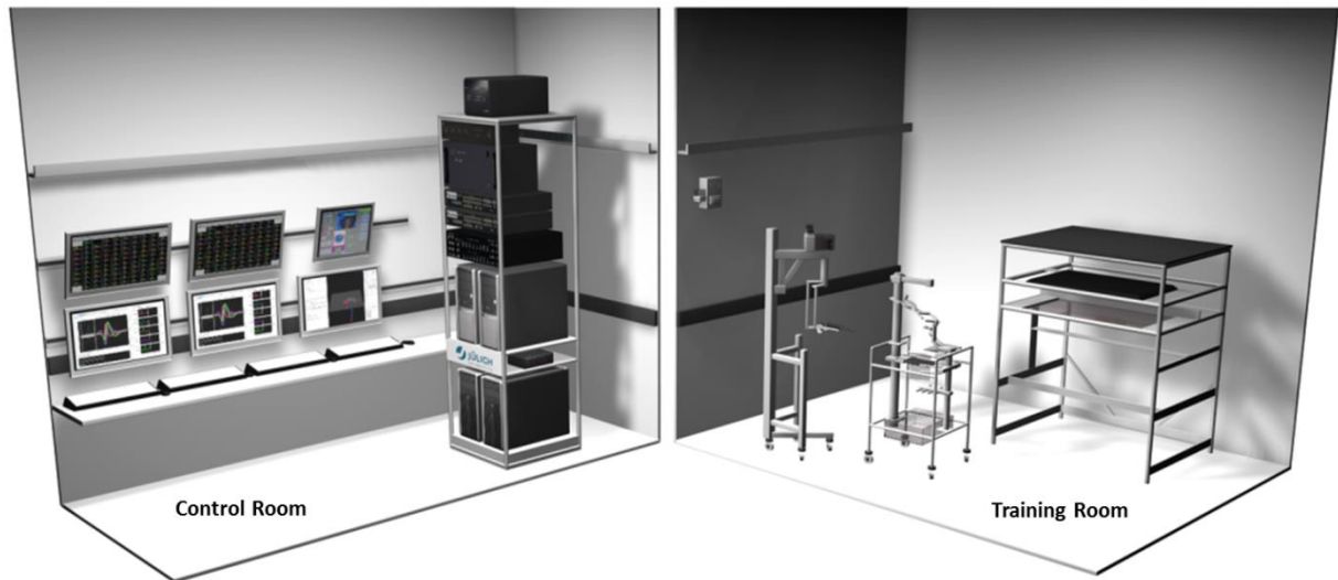
Figure 2.3: Control room adjacent to the monkey training room. 3D CAD design of the actual control and training room at the INT, deconstructed in Figure 2.4 into system components situated in both areas, featuring hardware connectivity and dataflow.
