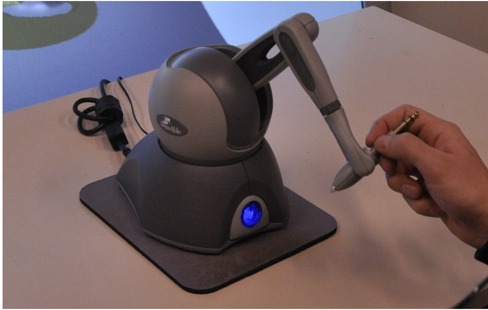
Figure 3.5: The Sensable PHANTOM Omni haptic device used in the study. To improve vibration forces, the plastic stylus cover was removed, and the device is gripped at the metal jack.
