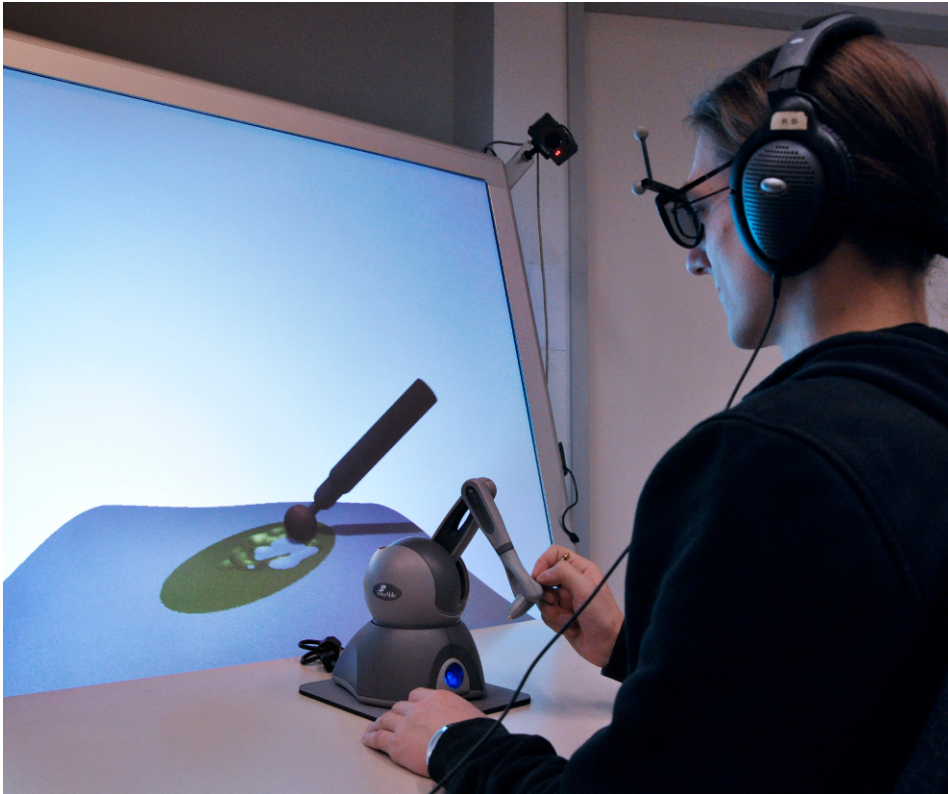
Figure 3.1: Setup of the study. The participant is seated in front of a stereoscopic scree, and uses a Senseable PHANTOM Omni to control a virtual drill in order to remove material from a surface.
