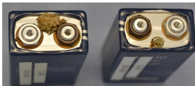
Figure 7.18: Salt deposition on top of the tested EDLC devices stored short-circuited at 65 °C (left) and 55 °C (right)
