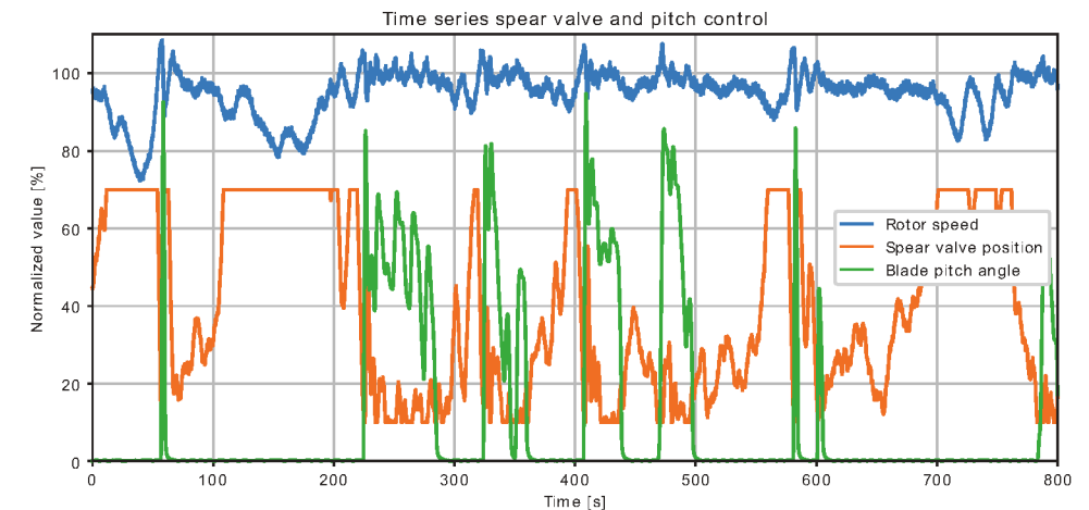
Figure 8: A time-series showing the hydraulic control strategy for the DOT500 turbine. The spear valve position (orange) actively regulates the rotor speed (blue) as a substitute to conventional turbine torque control. In the above-rated region, pitch control (green) is employed to keep the rotor at its nominal speed (100 %). All signals in this plot are normalized.
