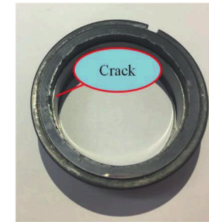
Figure 2 Fracture of stationary ring
