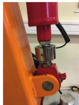
Figure 10. Force sensor for measuring payload
