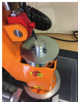
Figure 8. Rotary encoder for measuring base rotation
