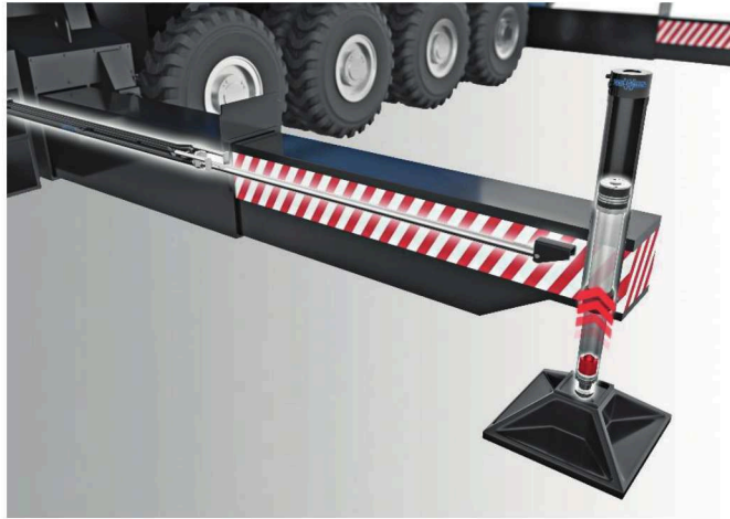
Figure 2: Supporting cylinder with integrated force measurement
