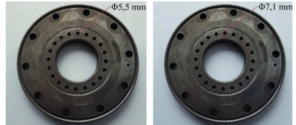
Figure 5: The minimal hole size ( \Phi 5,5 mm) in the valve plate ( \Phi 174 mm \times 15 mm). Figure 6: The desired maximal hole size ( \Phi 7,1 mm) in the valve plate ( \Phi 174 mm \times 15 mm).
