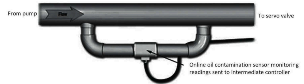
Figure 2: On-line continuous monitoring sensor connected to the pump delivery line.
