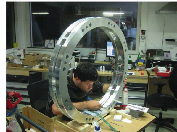
Figure 8: Torque sensor for 50.000 Nm with endstops during application of the strain gauges
