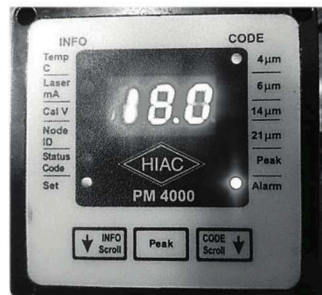
Figure 10: Alarm setting for 4\text{ }\mu\text{m} particles with target ISO code 18/16/13 according to ISO 4406.
