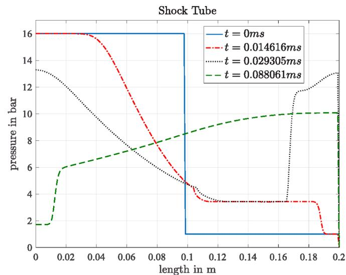
Figure 9: Pressure distribution of a closed Shock Tube.
