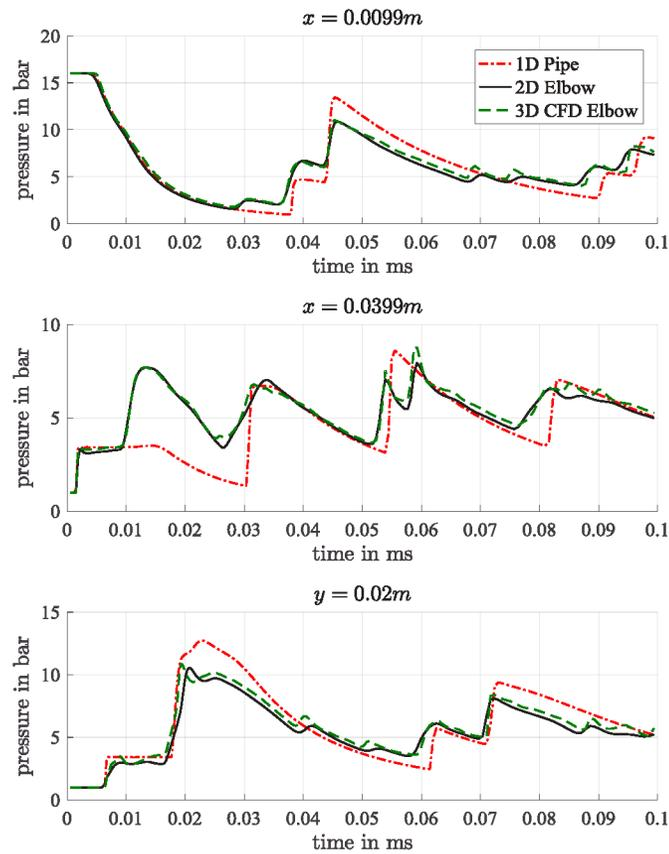
Figure 11: Comparison of 1-D, 2-D and 3-D CFD.
