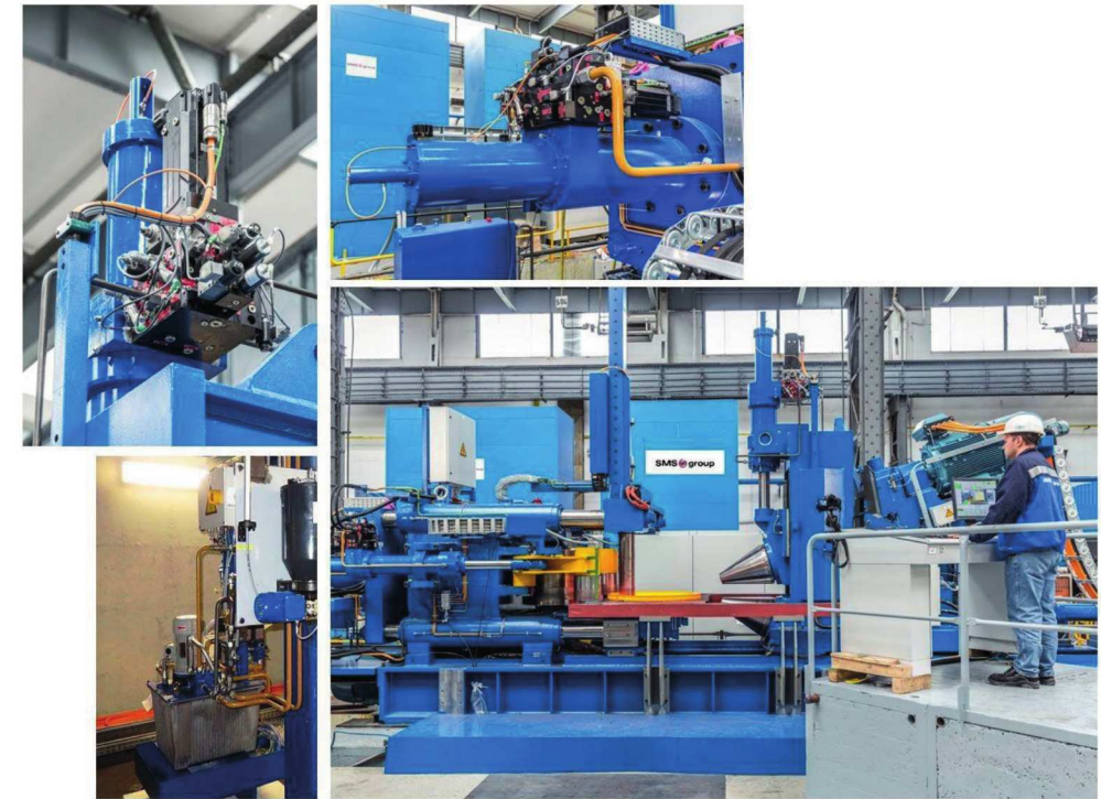
Figure 13: Ring Rolling Mill RAW ecompact, SMS group GmbH
