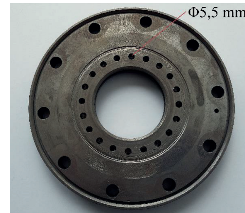
Figure 5: The minimal hole size ( \Phi 5,5 mm) in the valve plate ( \Phi 174 mm \times 15 mm).
