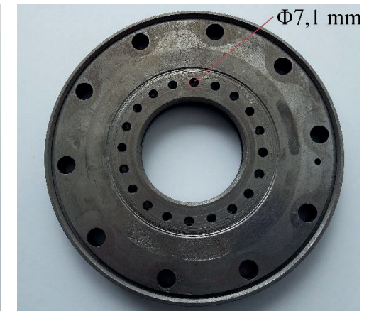
Figure 6: The desired maximal hole size ( \Phi 7,1 mm) in the valve plate ( \Phi 174 mm \times 15 mm).
