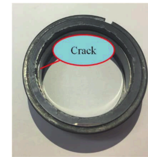
Figure 2 Fracture of stationary ring
