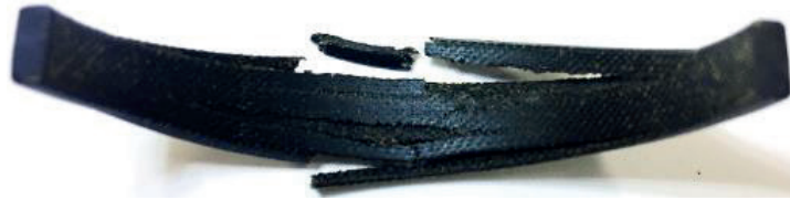
Figure 12: Test specimen fabric-base laminate with cracks
