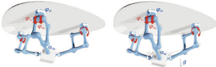
Figure 6-4: Available sensor information for the PARAGRIP handling system
