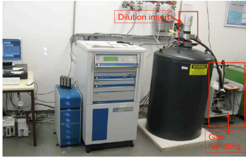
Figure 3.2.3 Photography of Quantum Design PPMS equipped with a dilution insert for low temperature heat capacity measurement. The dilution insert components are marked.
