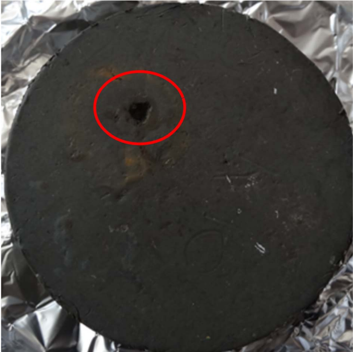
Figure 71: visual observation of sample K10: a piece of pyrite fell out of the sample, leaving a hole. Due to oxidation around that hole a brown zone was left behind, pointing to the presence of iron oxides.
