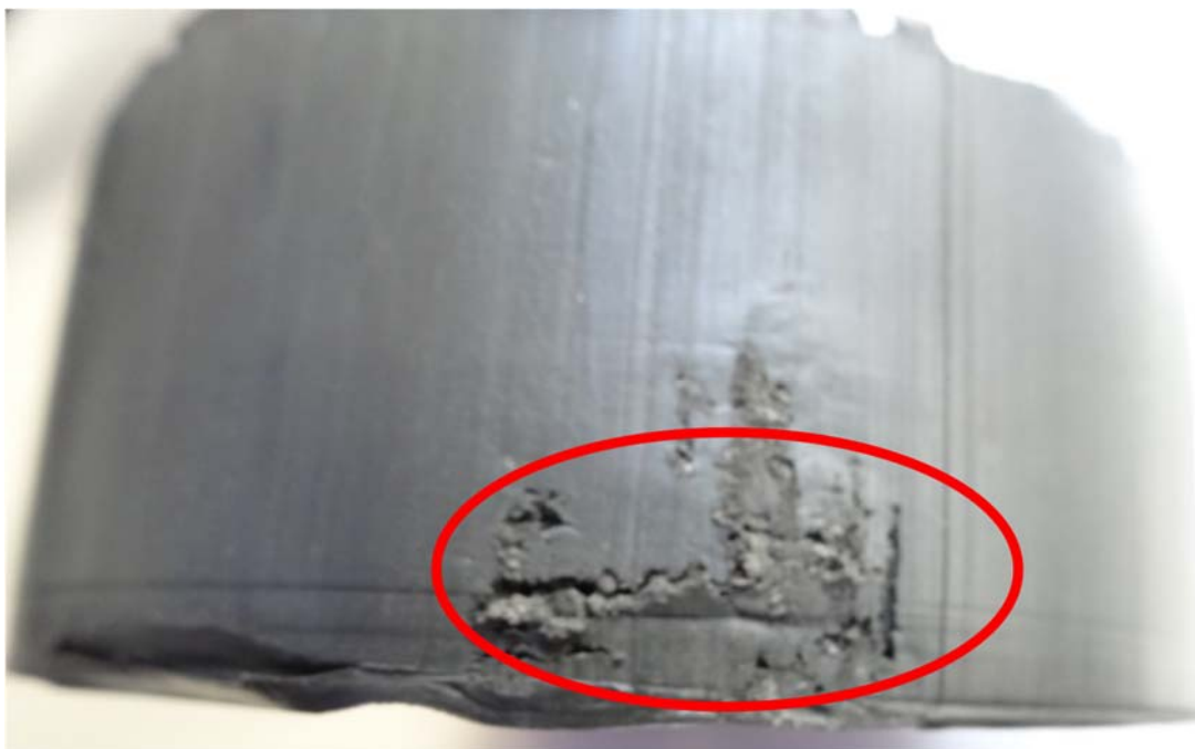
Figure 70: visual observation of pyrite in sample K4
