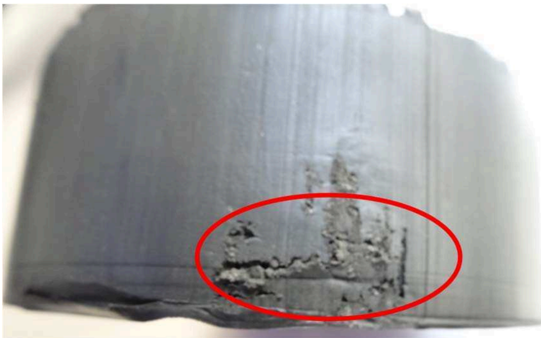
Figure 70: visual observation of pyrite in sample K4
