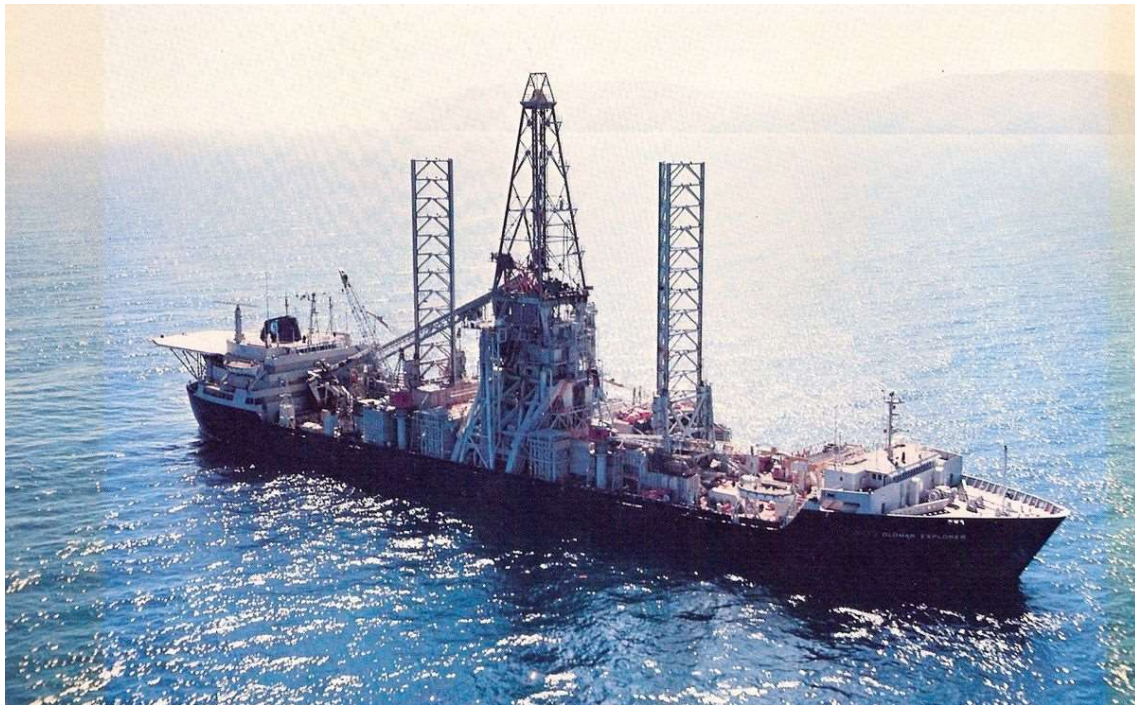
Figure 2.2. Photo taken from the Hughes Glomar Explorer employed by OMCO in 1976 and 1979 in the North Pacific. Although the vessel was scrapped, it would have met today's basic requirements for DSM (U.S. Government photo; published in Aid et al. 2010).
