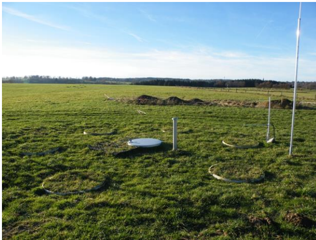
Figure 3.1: The lysimeter set-up of the Rollesbroich study site (November 2012).
