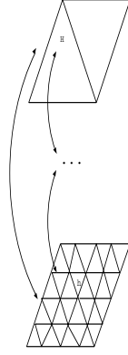
Figure 9.5: All elements of the finest grid have links to the elements of the coarsest grid and vice versa.
