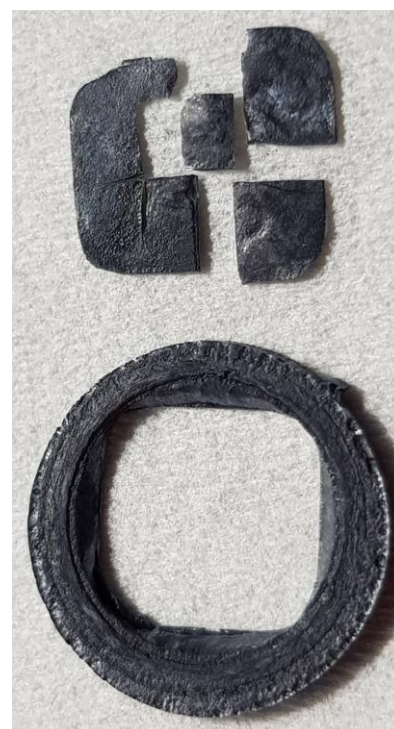
Fig. 44: Second discharge current/voltage profile of Si-air cell 13 during in-operando NMR and photograph of the Si-wafer anode after discharging. Left: The second discharge test of cell 13 was performed after complete recovery of the cell voltage, which broke down at the end of the first test (Fig. 43). After decreasing the electrolyte flow rate to approximately 0.01 \text{ ml} the cell voltage decreased. By increasing the flow rate stepwise a discharge voltage of around 1 \text{ V} for a flow rate of approximately 0.5 \text{ ml/min} was found. The corresponding in-operando ^{29}\text{Si} NMR measurement is shown in Fig. 45. Right: The photograph shows the Si-wafer anode after the end of discharging for cell 13. The (almost rectangular) parts, shown at the top, were such thin that they broke apart from the remaining Si-wafer, shown at the bottom. Thereby the active surface of the Si-wafer surface changed and strong fluctuations of the cell voltage were observed in the last 5 h of discharging.
