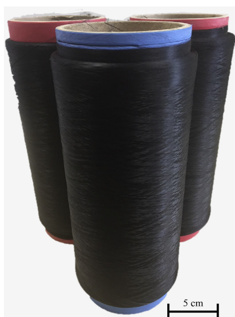
Fig. 2. Examples of graphene-modified PA6 multifilament yarn bobbins. (A colour version of this figure can be viewed online.)
