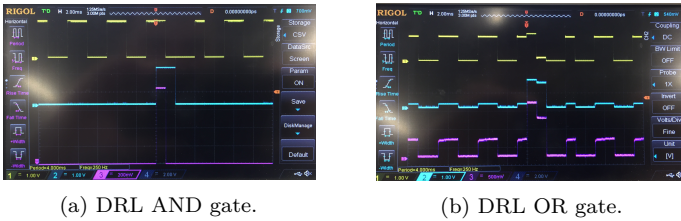
Figure 4.19: Oscilloscope captured inputs and outputs of the fabricated DRL boolean logic gates.
