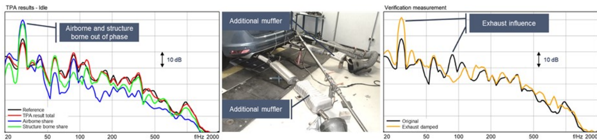
Figure 7 - TPA model verification by modification measurements
