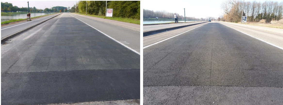
Figure 2 – The test track: on 8 October 2018, just after completion (left) and 4 months later, on 29 February 2019 (right). Some slight “general” ravelling is noticeable.
