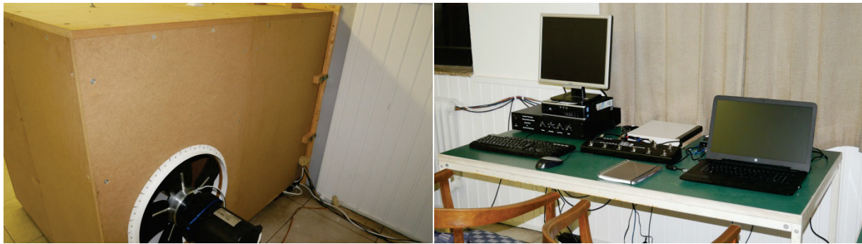
Figure 3 – Infrasound source with the TRW-17 (left) and the control / measurement devices (right)
