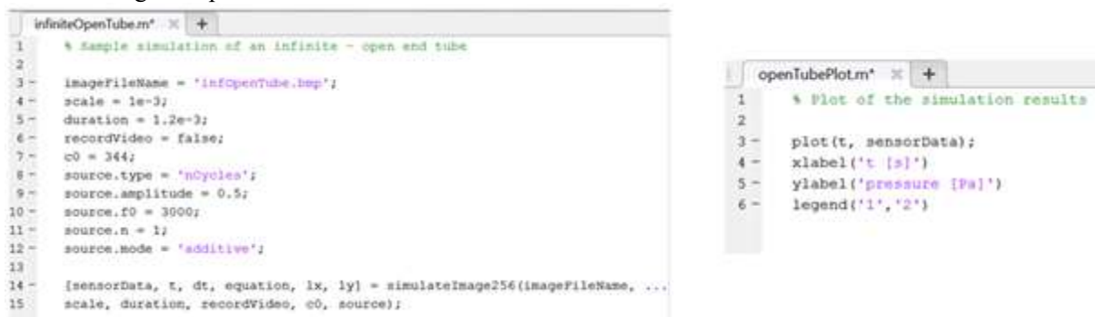
Figure 9 –Sample code for the simulation of an infinite tube with an open end
