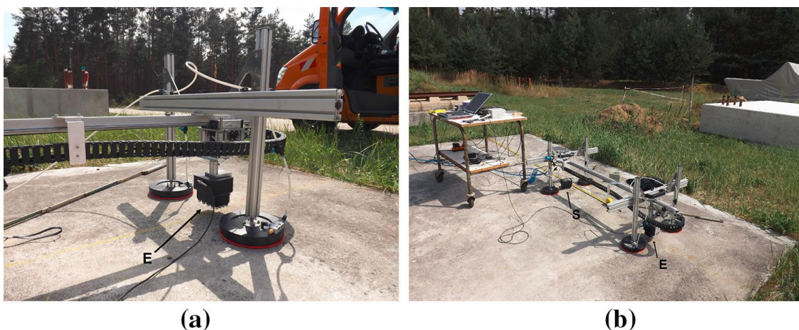
Figure 5-27: (a): Scanner on the foundation slab moving the receiving transducer array (E) and (b): scanner with transmitting (S) and receiving (E) transducer arrays.
