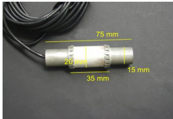
Figure 4-5: Photograph of the novel ultrasonic transducer for embedment in concrete (Manufacturer: ACS Ltd., Moscow, Russia. Photo: BAM).
