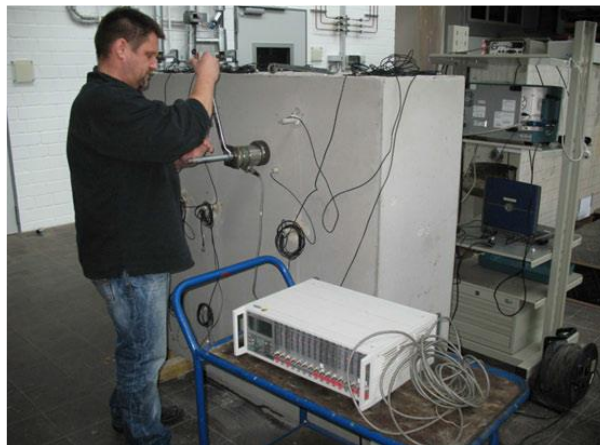
Figure 4-14. Concrete specimen GK32 with embedded transducers and load application system. From Niederleithinger et al. (2014).
