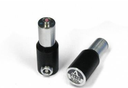
Figure 4-2: Point contact ultrasonic transducers as used in most state of the art devices for concrete (Low-frequency transducer S1802, shear waves, 50 kHz, ACS Ltd.)
