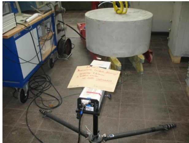
Figure 4-10. Experimental setup for measurement of directivity patterns. Transmitting transducers are embedded in the center of the concrete block. Surface movements are recorded by a laser vibrometer (in front).
