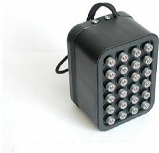
Figure 4-3: Ultrasonic array with 24 transducers of the type shown in Figure 4-2. The upper four by three are directly coupled and work a transmitter array, the lower four by three as a receiver array. (ACS Ltd.)
