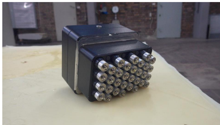
Figure 5-26: Ultrasonic transducer array consisting of 32 dry point contact transducers
