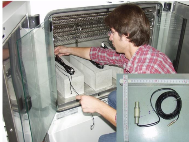
Figure 6-5: Climate chamber with samples equipped with embedded ultrasonic sensors. Lower right: sensor before embedment.
