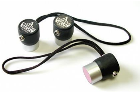
Figure 4-1: Conventional ultrasonic transducers for concrete investigations (Low-frequency transducer S0208, longitudinal, 100 kHz, ACS Ltd.)
