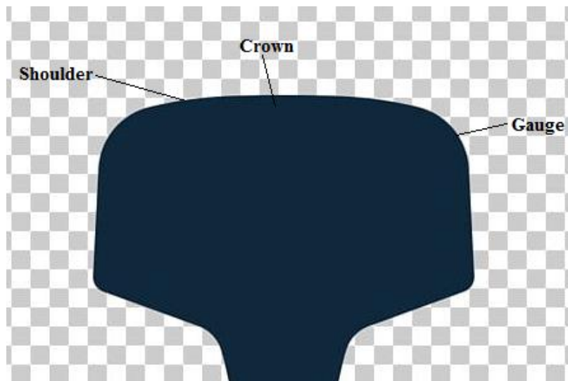
Figure 4: Rail profile is classified into- Rail shoulder, rail crown and rail gauge
