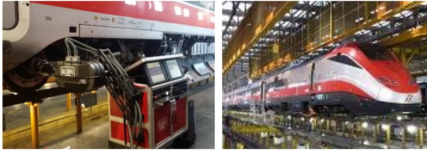
Figure 39: UT bore-probe inspecting an axle of a trainset in the depot.
