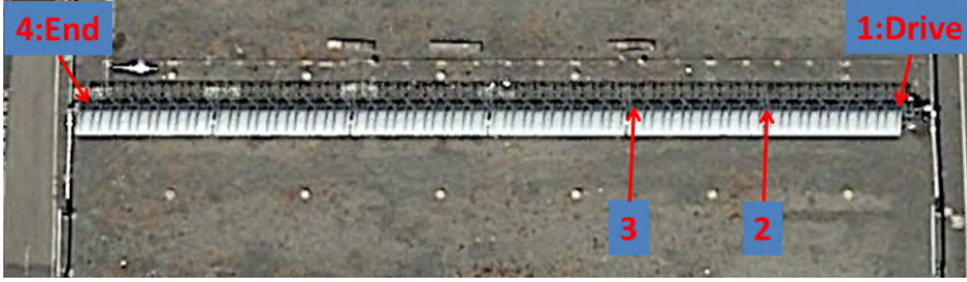
Figure 3.13: Google maps view on the east-west orientated EuroTrough (ET) prototype SCA at the PSA. The SCA extension in east west direction is approximately 70 m, which corresponds to a total number of six SCEs. Inclinator assemblies have been attached to the drive (1), to the FEP of the 2 nd SCE (2), to the REP of the 2 nd SCE (3), and to the REP of the 6 th SCE (4).
