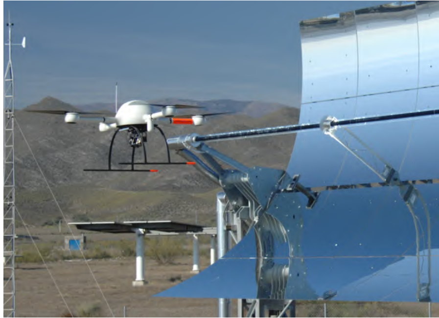
Figure 4.2: Microdrones md4-1000 during a test flight in front of the KONTAS test facility at the PSA.
