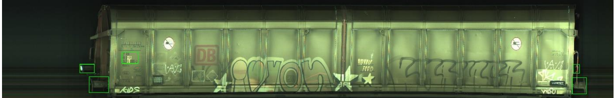
Fig. 2 Upper image of cargo wagon. Green rectangles are labels of bumpers and UIC ID
