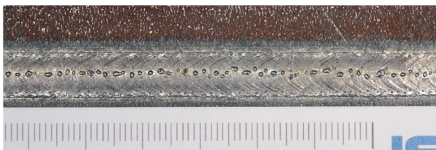
Fig. 11 Weld bead appearance of S960M mill scale-covered sample
