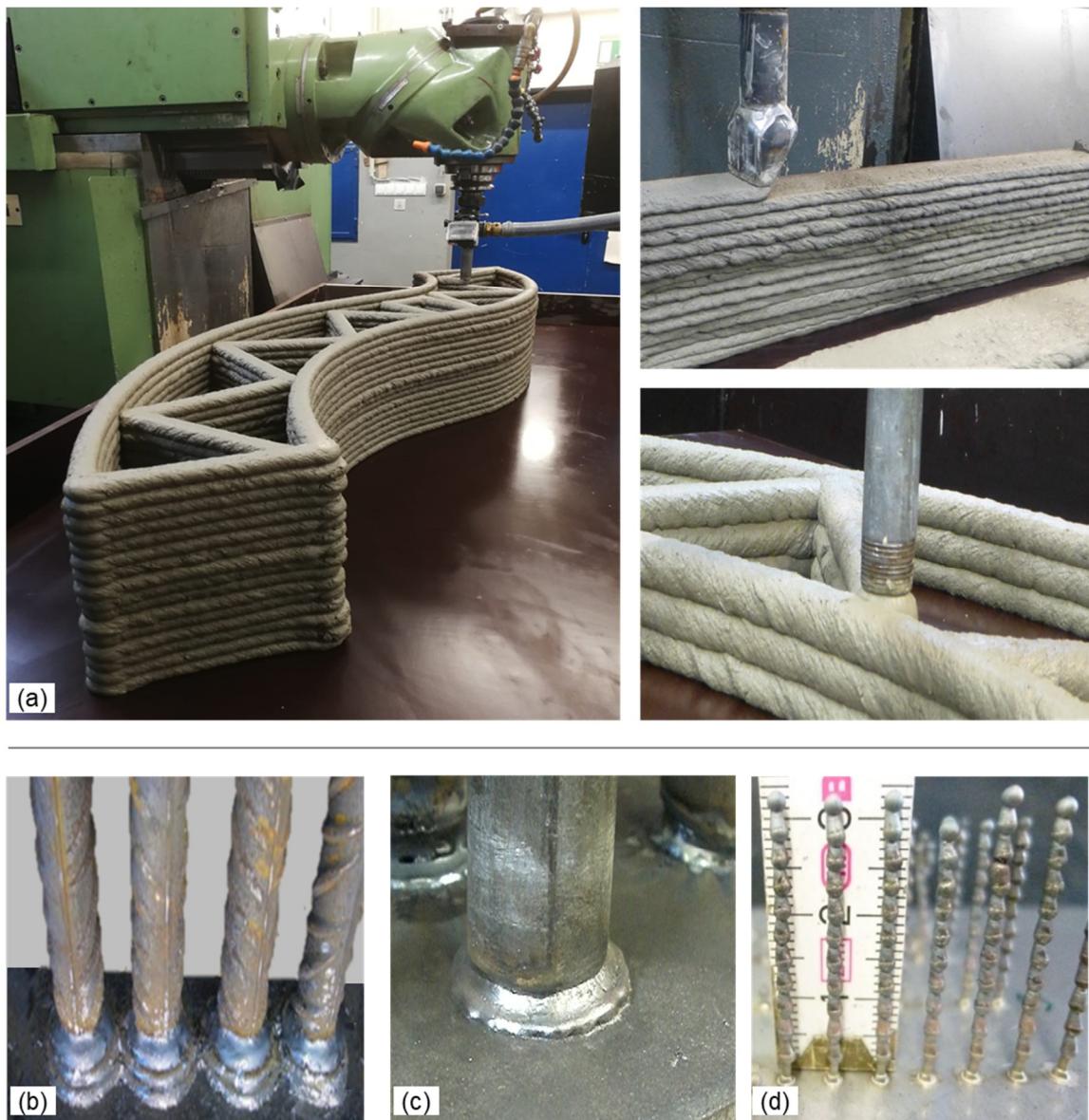
Figure 3. 3D printing of a non-reinforced demonstration objects at Institute of Structural Concrete of RWTH Aachen University (a), preliminary work for joining of reinforcement and additive manufacturing of steel at Institute for Joining and welding technology of RWTH Aachen University: MAG welding (b), stud welding (c), pin welding (d).
