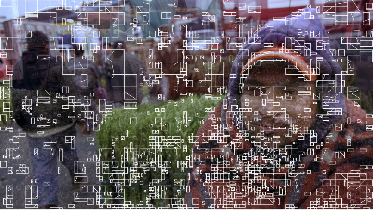
Figure 5.8 Picture with highest maximum memory bandwidth increase measured for the entire test set at 18.32% compared to the VTM-3.2 anchor. In this particular example of the MarketPlace sequence (POC 532) coded at QP22, a scene transition occurs in combination with object motion (persons on the left and right) and also dynamic texture motion (plants), causing a high usage of bi-prediction and geometric partitioning at the same time. The usage of GEO in this picture is 31.04% in terms of pixels coded.
