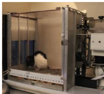
Figure 2.2: Touchscreen Chamber by Leising et al. 2013. The rectangular area for rats is shown. On the right side, the reward delivery system is visible. The screen on the left side is an attached Apple iPad
