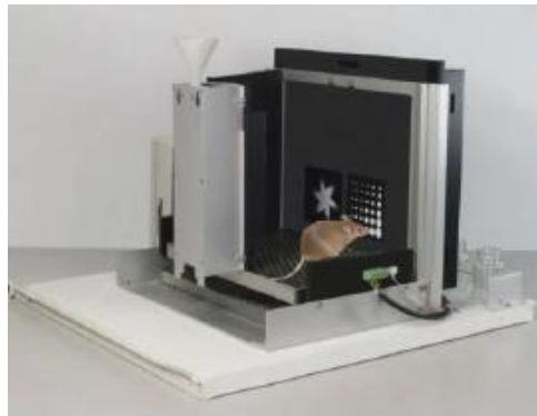
Figure 2.5: Bussey-Saksida Touchscreen Chamber (Horner et al. 2013). An opened touchscreen chamber is shown. In the experimental setting, the open side is closed. The reward delivery system is shown as well as the touchscreen. The area of the touchscreen, which does not show the stimulus is masked.
