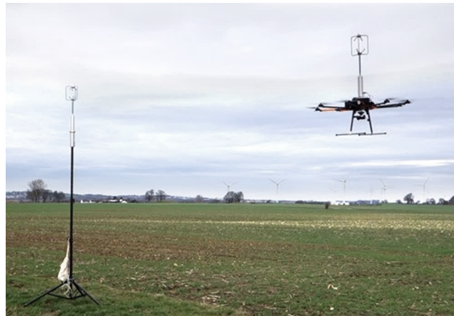
Figure 5. WindLocator hovering close to stationary anemometer.
