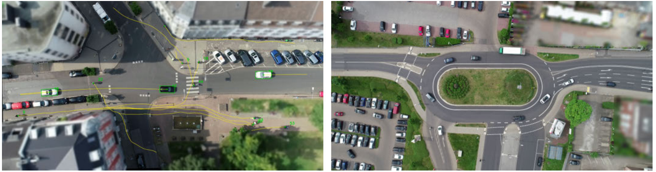
FIGURE 7. Scenes of real-world data recorded utilizing a drone: Road network of an intersection (left hand side) with marked trajectories of road users (yellow lines) and a roundabout (right hand side). Buildings are blurred in the recordings in order to meet regulations on privacy of information.
