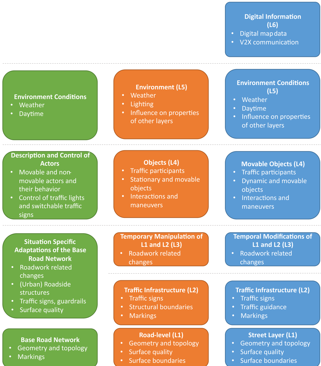
FIGURE 1. Historic development of the 6LM. Four layers of Schuldt [16] (left) compared to the five layers of Bagschik et al. [17] (center) and the six layers of Bock et al. [18] (right).
